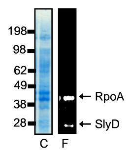
**Figure S1 TRAP labeling of CCPGCC-tagged RNA polymerase alpha (RpoA) in** *S. oneidensis.* TRAP-labeled RpoA was labeled in living *S. oneidensis.* An aliquot was harvested prior to photoactivation, lysed and run on an SDS-PAGE gel (4-12% bis-tris, Invitrogen), and visualized using fluorescence (F; ex: 465 nm, em: 535 nm) or scanned after staining with Coomassie blue (C). The two bands in the fluorescence image are tagged RpoA (runs at 42 kDa) and SlyD (runs just below 28 kDa).
